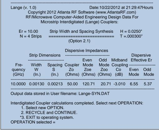
Figure 4-1: Typical Output Data for **Dimensional Synthesis** from Lange.exe
