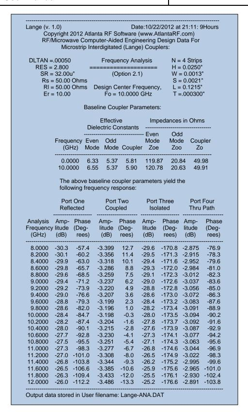
Figure 4-2: Typical Output Data for **Frequency Analysis** from Lange.exe
